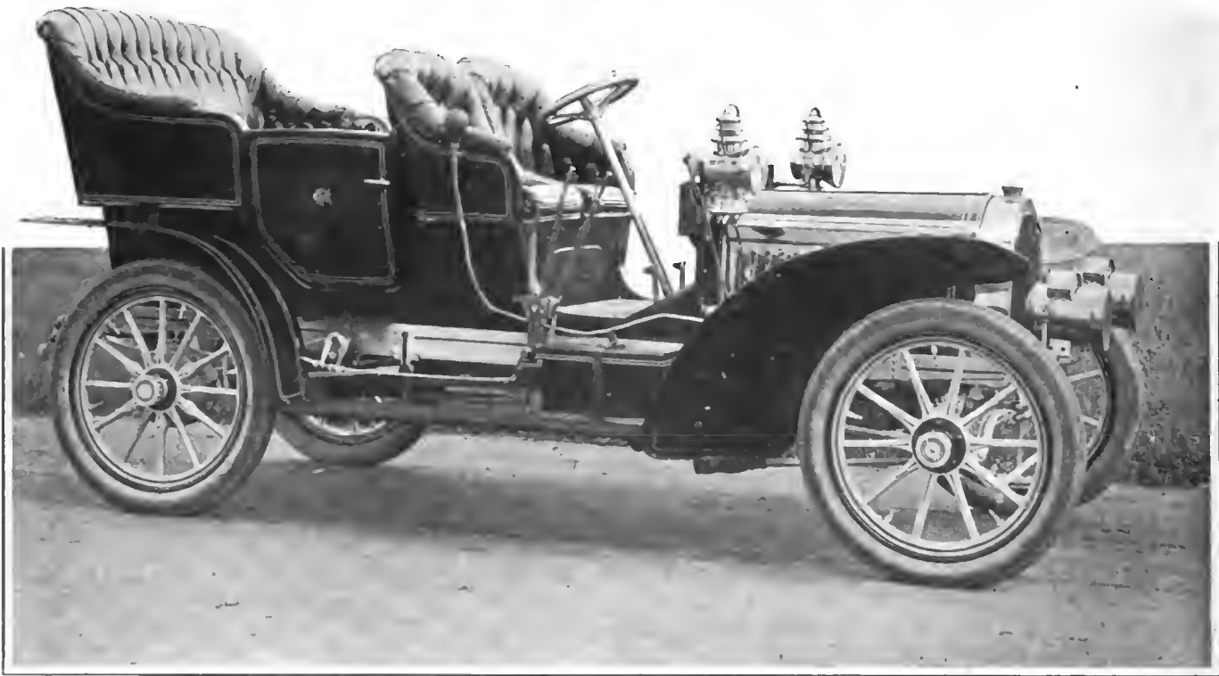
NEW 1905 MODEL N PACKARD 22-28 HORSEPOWER TOURING CAR, WITH SIDE ENTRANCE TO THE REAR SEAT.
